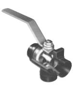
Victaulic Series 723 Diverter valve is a NACE MR-01-75 compliant three-port ball valve with common bottom inlet for diverting flow 90° left or right. 180° operation is optionally available. This valve is rated for 600 psi (4135 kPa) service.
