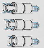
Within operating pressure differential range, the effective open orifice area of the cartridge is automatically adjusted to the point where the specified flow rate will be delivered (as the pressure differential increases, the open area closes and as it decreases, the area opens).
