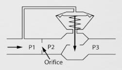
For the FlowCon A/AB/ABV, the principle of operation is shown above and the principle of construction is shown below. P1 and P3 are system pressures, P1÷P3 is the total pressure drop across the valve. P2 is set by the diaphragm acting in reaction to P1 in the upper diaphragm chamber. Interacting with the spring, P1÷P2 remains constant, keeping a constant  $\Delta P$  across the orifice areas. The result is a constant flow rate through the valve, independent of pressure fluctuations.
