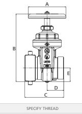
Straightway pattern, non-rising stem, 300 lb. hose gate valves are intended for use on standpipes, fire pumps and hydrants.
