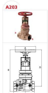
400lb. field adjustable automatic pressure regulating valve for use as a fire hose rack assembly valve or sprinkler control valve where pressure requires regulation.
