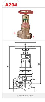
400lb. field adjustable automatic pressure regulating valve for use as a fire hose rack assembly valve or sprinkler control valve where pressure requires regulation.
