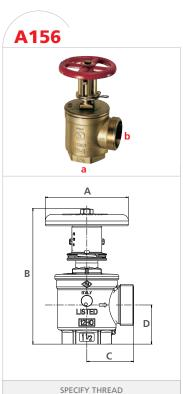
Adjustable restriction of residual pressures up to 175 lb. Locking pin device restricts full opening of valve by untrained personnel, pin may be removed by firefighters to allow full opening of valve.
