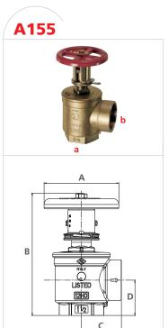
Adjustable restriction of residual pressures up to 175 lb. Locking pin device restricts full opening of valve by untrained personnel, pin may be removed by firefighters to allow full opening of valve.
